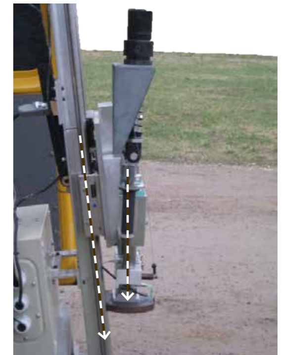
▲ The metal “hoof” is mounted beneath a heavy weight, which is dropped to the ground between two guide rails. The rails have different angles, which mimics the motion of the early landing/touchdown phase, as a simultaneous downward motion and forward slide of the ‘hoof’ occurs when it contacts the ground.
