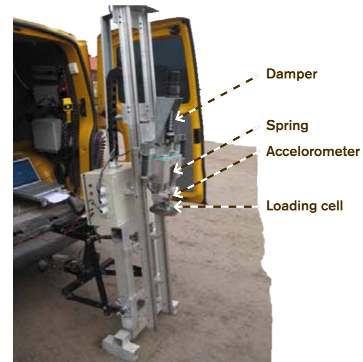
▲ The Orono Biomechanical Surface Tester simulate the impact of a horse’s leg on the ground. The machine is mounted at the back of a van or truck of sufficient weight, for ease of transport between and on arenas, and is supported by a frame, which is placed on the ground for stability during testing.
